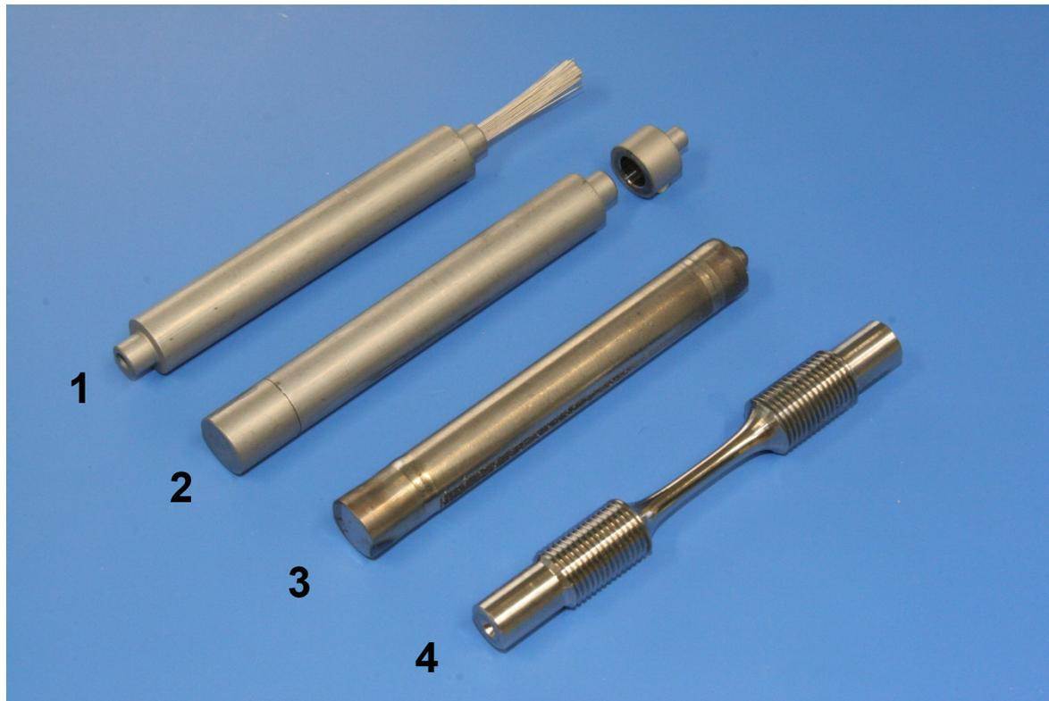
1. Bundle of coated fibers to be filled into especially designed component (lengthwise / spooled depending on direction of load)
